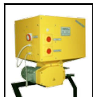
**FEATURES:** Compact and solid design, maximum efficiency in small spaces and easy to use. Upper cereals container (**capacity 136 L.**), discharge hopper, its own stand, a switch safe-motor and patented wear-resistant rollers. The crusher rollers are treated with a wear-proof coating that makes them very resistant. The machine does not produce dust, is silent and has no vibrations. One-year warranty.
