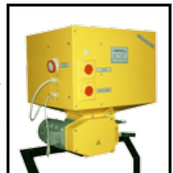
**FEATURES:** Compact and solid design, maximum efficiency in small spaces and easy to use. Upper cereals container (**capacity 90 L.**), discharge hopper, its own supporting trestle, a switch safe-motor and patented wear-resistant rollers. The crusher rollers are treated with a wear-proof coating that makes them very resistant. The machine does not produce dust, is silent and has no vibrations. Two-years warranty.
